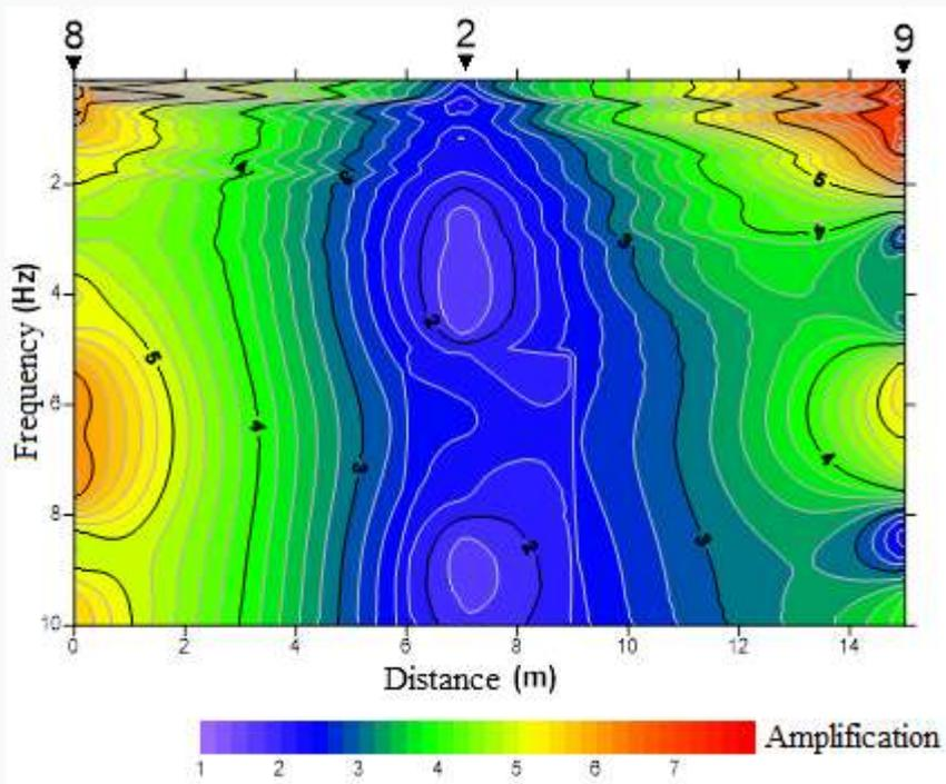
Figure 10. Spatial analysis of path A with 3 measurement points, at point 8, 2 and 9.
