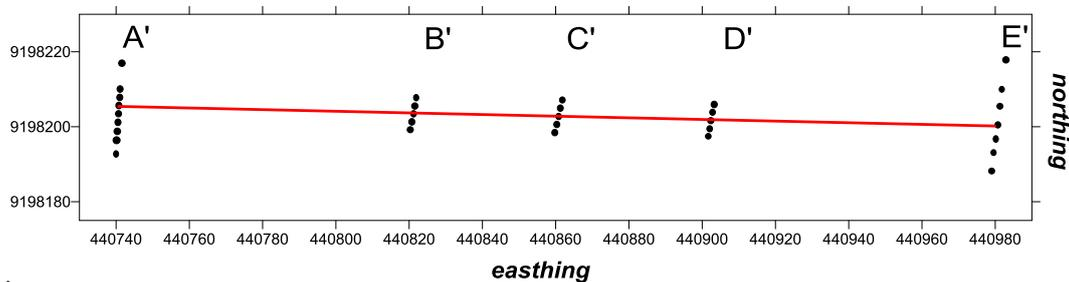
Figure 8, The pipe line indication is marked with a red line extending from line A to line E
